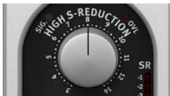
Scale values for the filter are displayed in dB. The actual reduction values, i.e. after phase cancellation, are displayed in the upper SR LEDs. Thus, when the control is set to 3 dB, actual reduction might only be of around 1 dB. The SR LEDs display sibilance reduction between -1 dB and -14 dB, first in 1 dB increments and from 6 dB on in 2 dB increments. Please note that the MALE/FEMALE button has no effect on the high-band de-esser.
