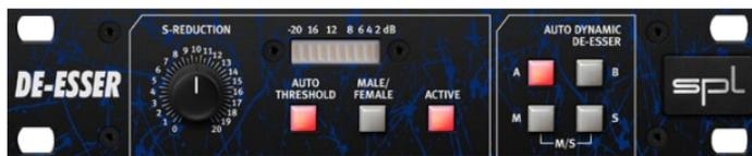
Back in the 1990's, we developed an alternative way to process signals in order to reduce sibilance based on phase cancellation. Unlike traditional compression methods, this procedure is much more unobtrusive and simplifies control to one single parameter. SPL's De-Esser quickly became a standard reference among recording studios, broadcast stations and live sound engineers.
